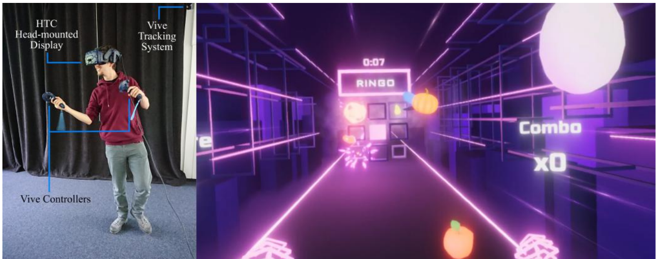
Figure 1: Experiment setup. Subject wearing the HMD with controllers (left), and a picture of the corresponding gameplay.
