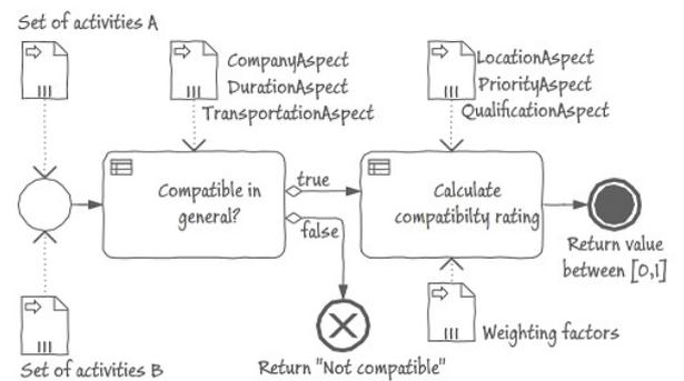
Figure 5: Conceptual process of the calculation of the compatibility rating as BPMN diagram
