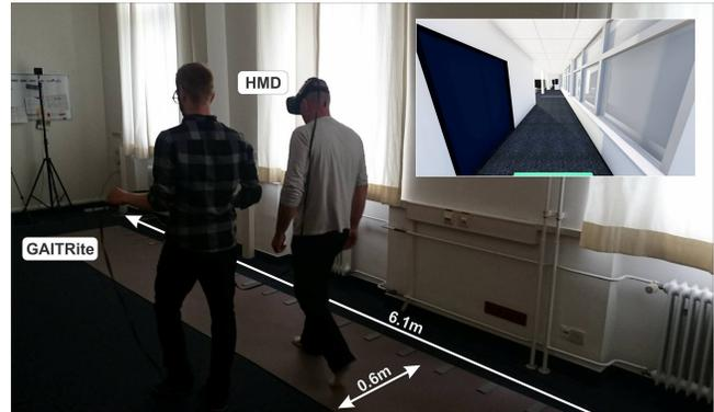
Figure 1: A participant walks with an HMD over the GAITRite walking surface; the inset shows the participant’s view on the HMD.
