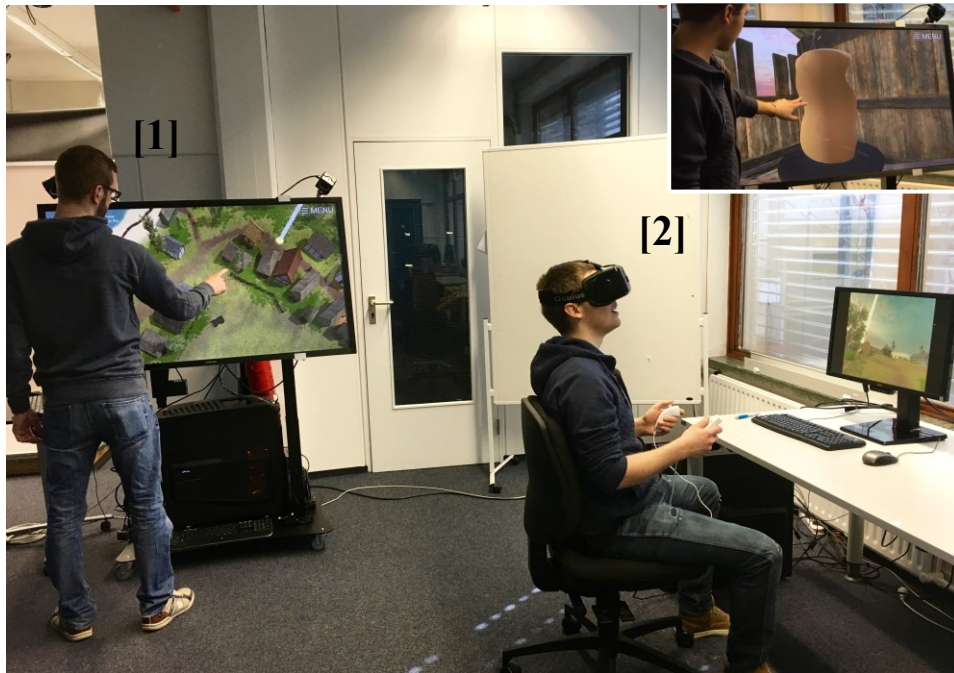
Figure 1: Illustration of the setup of the multi-user interactive exhibition. Player [1] is using the multi-touch table and player [2] is wearing a head-mounted display. Both players are present in the physical setup while experiencing the same shared virtual space from different viewpoints. (Note that the distance and angle of users is just for photographic reasons. Usually users cannot see the screen of the other player). The inset shows a user performing the virtual pottery task using touch input to form virtual clay.
