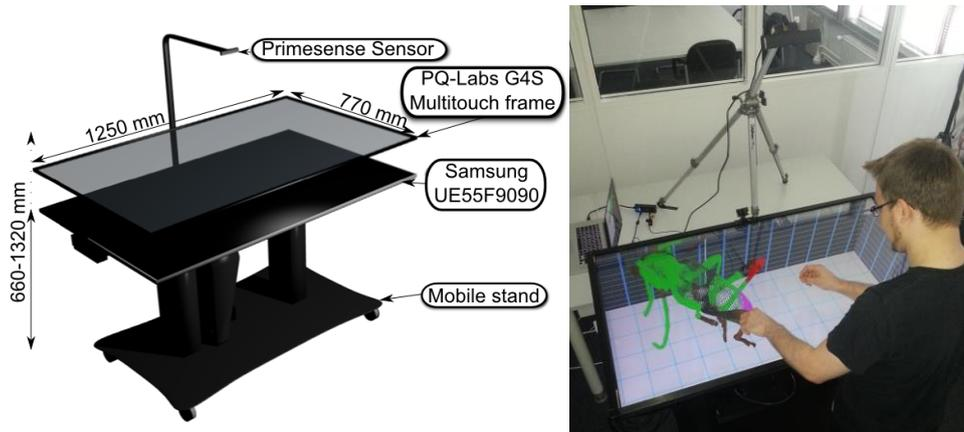
Figure 1: a) Schematic illustration of the interactive Spatial Surface in the tabletop mode. b) Illustration of work at the interactive Spatial Surface for annotating a point-cloud data set (Headtracking marker at camera position)
