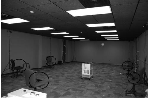
Figure 1: Multiple Kinects are arranged in a circular manner. Circled Kinect is the primary tracker. Kinects circled with dotted lines are providing IR interference.
