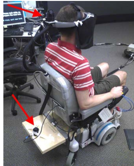
Figure 2: Here is shown the dual tracker setup used to differentiate the subject's head motion from the motion of the wheelchair. The wheelchair and head motion is used for rendering the virtual scene, and the wheelchair position is used in the PID steering controller.
