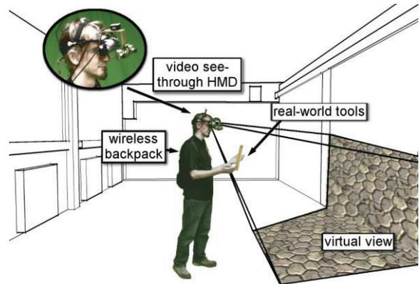
Figure 1. Illustration of the virtual studio environment: The frustum on the right illustrates the user's view of a virtual scene, while the video see-through HMD captures real-world tools and objects, which are displayed in the mixed-reality view on the HMD; the left inset shows a modified eMagin Z800 HMD with attached cameras and sensors.
