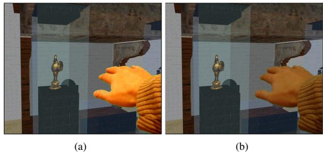
Figure 3. Composition of pixels corresponding to a user's arm and hand with a view to a VE (a) without and (b) with brightness adaptation.
