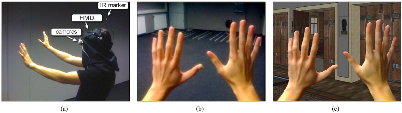
Figure 1. Virtual body in an augmented virtuality scenario: (a) user in a video-see-through HMD setup; cameras attached to an eMagin 3DVisor Z800 HMD at approximate eye positions. (b) Camera images showing the user's hands in the real world and (c) the user's virtual view with the segmented hands.
