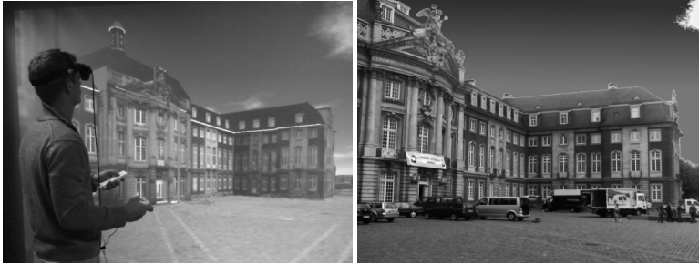
Figure 1: (left) Multimodal locomotion setup consisting of HMD, optical tracking system, and Wii. The projection wall illustrates the user's view. (right) Photograph of the same building.
