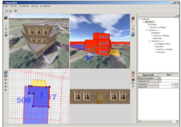
Figure 3: A screenshot of the two-dimensional building editor mode. The two-dimensional frames are displayed monoscopically, whereas the previews of the three-dimensional building can be displayed stereoscopically.
